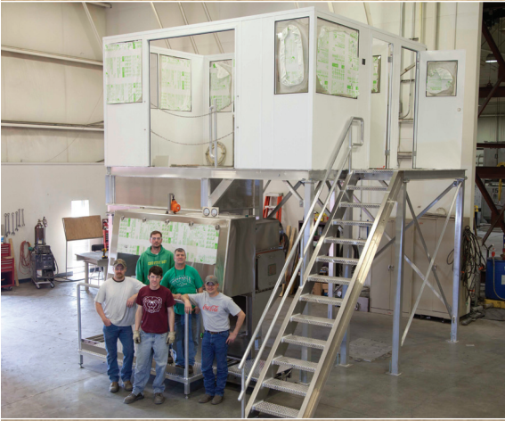
Integrated Station for Drum Discharge, Product Milling & IBC Loading
