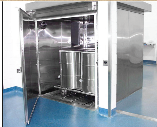
Drum/IBC Washer, Pass Through Wall Configuration
