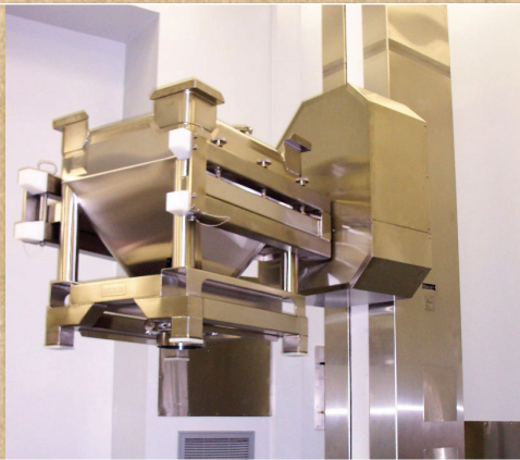
Column Blender with Lift, Blend, Slew & Invert Capability
