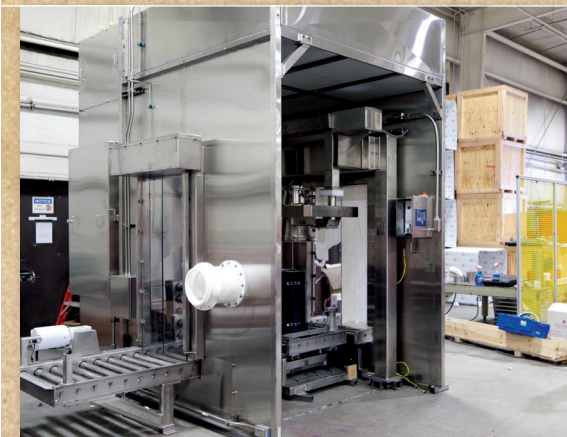
Downflow Booth for Drum Delidding & Containment Discharge
