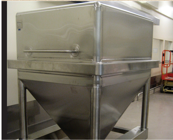
IBC Transfer Bin with Casters & Forklift Channels
